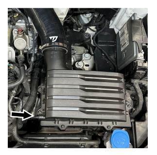
17. All the clamps can now be tightened using the 7mm socket or flathead screwdriver, and the air duct can be reassembled.
