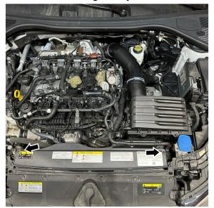
3. Unclip the air duct vent from the air duct and remove the vacuum line that runs from the intake to the manifold to the airbox
