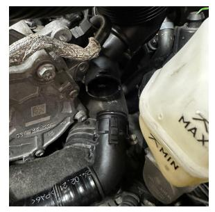
6. Using your 7mm socket or flathead screwdriver, loosen the clamp on the intake tube to the turbo inlet elbow and remove the intake tube or entire airbox from the engine compartment.
