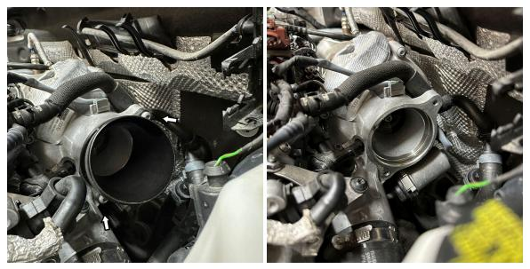
8. Open the hardware kit provided with your turbo inlet elbow (UH045-IN0) and install the provided o-ring onto the inlet elbow (UH020-IN8)
