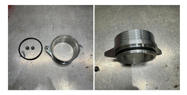
9. Install the Unitronic turbo inlet elbow onto the turbocharger. A little bit of silicone lube will help with the installation of the new O-ring. Note:The Unitronic "U" Logo will face towards the top of the turbocharger.
