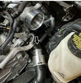
12. Locate the Silicone intake hose upgrade (UH43-IN2), one of the large hose clamps, and the small clamp provided, and place the small clamp onto the silicone hose. This will be used to secure the aluminum adapter installed in step 12 to the silicone hose. The orientation of the clamp is important as it will need to be fastened in place when the silicone hose is installed onto the turbo inlet with minimal access.
