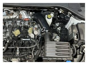
16. If the factory airbox is used, a vacuum port plug will be required (Not included) to plug the intake manifold runner flap vacuum line.
