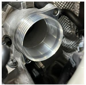
11. With the Unitronic Silicone Intake hose, there will be an aluminum adapter. This adapter will be placed onto the Diverter Valve tube. There are two grooves that the adapter will fit into. Push the adapter onto the diverter tube to secure it into place.
