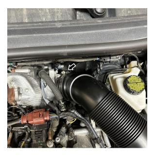
7. Using a T30 Torx bit and extension, remove the two (2) fasteners holding the turbo inlet elbow to the turbocharger
