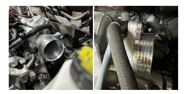
10. Using the provided 4mm fasteners, install both fasteners into the inlet elbow to secure the elbow to the turbocharger.
