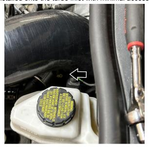
13. Using the 7mm socket or flathead screwdriver, fasten the small hose clamp that will secure the aluminum adapter into the silicone tube. The larger hose clamp on the turbo inlet can remain loose until the Air box is reinstalled.
