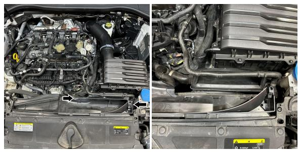
4. Carefully lift the Air intake box by pulling it upwards. It is important not to remove the entire box from the engine bay at this point. The diverter valve tube will need to be disconnected from the bottom of the intake tube. You may also remove the clamp on the intake tube and remove only the airbox leaving the tube in place.
