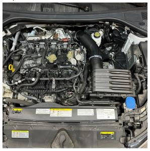
2. Using a T25 socket, loosen the two (2) fasteners on either side of the air duct and remove the air duct cover from the engine bay.
