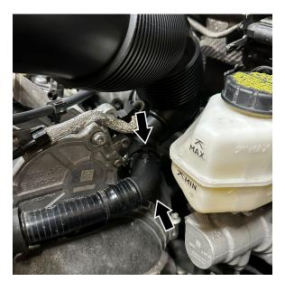
5. To remove the Diverter tube from the intake tube, push down on the upper and lower tabs and pull outwards.
