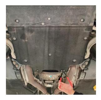
16. Reinstall the engine heat shield with 4X13mm ball studs.
