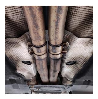
7. On both sides remove the bolt and spring fastening the mid-pipes to the adjustable bracket using a 13mm socket.
