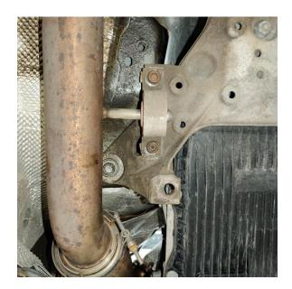
14. Reinstall the exhaust slip-on clamps connecting the mid-pipes to the exhaust system using a 13mm socket.
