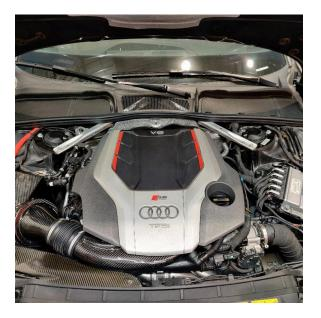
3. Remove the 4 ball studs from the engine heat shield as shown using the 13mm deep socket.
