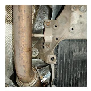
9. Now the V-Band clamp can be loosened with a T30 TORX socket and the clamp removed. Pull the OEM downpipe up and away from the firewall carefully.
