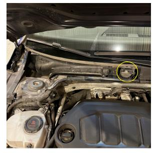
6. Under the soundaktor, there is a 6-pin connector with a locking tab. This will be difficult to remove since the locking tab will need to be unlocked before the connector can be removed. To unlock the tab, it will need to be slid towards the right side of the vehicle (Driver Side). A 90 Degree pick can be used to unlock the tab.
