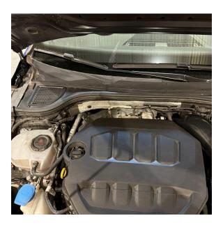
2. Remove the weather stripping on the rain tray
