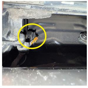
7. With the 6-pin connector removed, locate the UH037-FL7 (Unitronic Feat Box Wiring Harness). This harness will have three Connectors.
