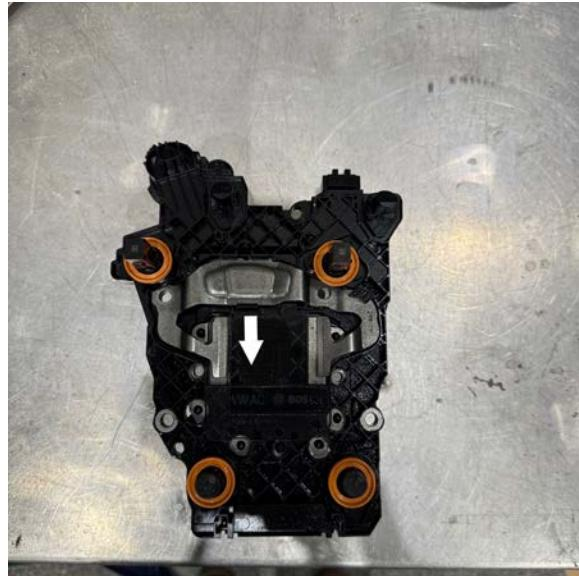
18. Place the clutch pressure sensor plate onto the replacement TCM by first sliding in the right side of the plate under the tab shown in the photo below, then push into place, ensuring that the plate clips in and is 100% seated
