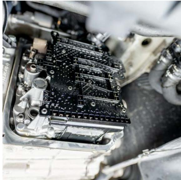
14. With the mechatronic placed on a clean workspace, remove the twelve (12) T20 torx fasteners from the front side of the mechatronic unit and remove the plastic cover by pulling up on the plate. This plate is connected to the mechatronic and the TCM. Use even force when removing the plate from the mech unit.
