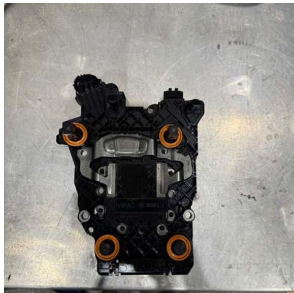
19. The replacement TCM may require you to transfer your (orange) seals from the original TCM. Take note of the fully seated orientation BEFORE removing them from the original TCM. Be sure to transfer these over in the correct orientation BEFORE proceeding to the next step.
