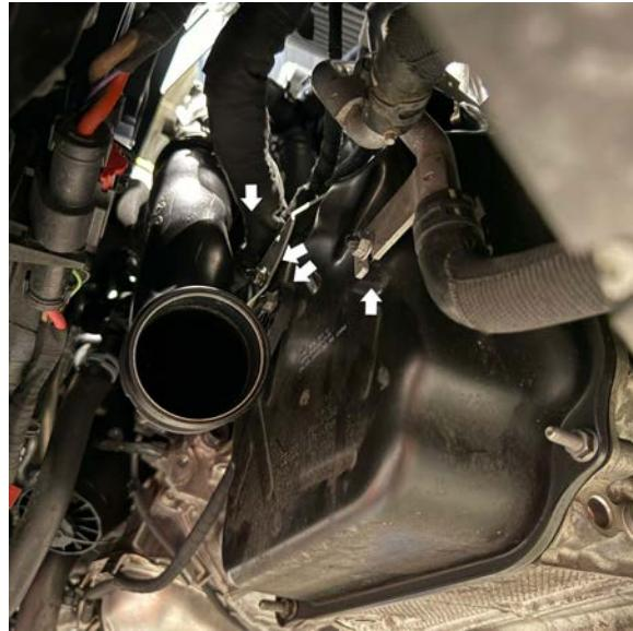
7. Disconnect the TCM connector by turning the locking tab counterclockwise (to the left). Once turned, the connector must be pulled towards the front of the vehicle.
