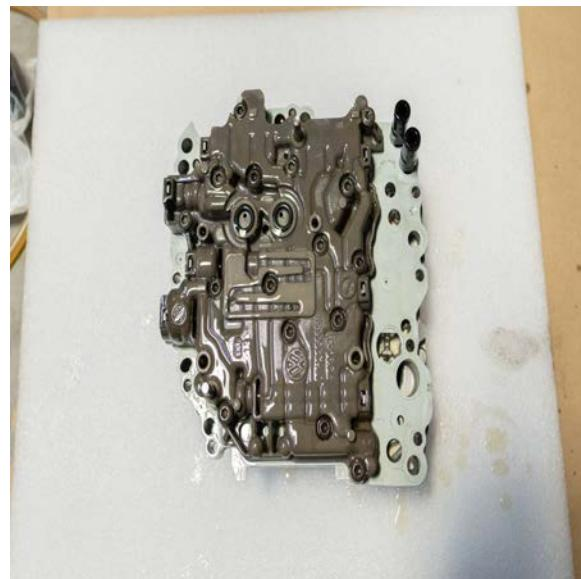
17. Some TCMs may not come with the Clutch Pressure Sensor Plate installed. This will require you to swap the CP plate from your existing TCM to the new unlocked TCM. To remove the plate, use your finger to push down on the tab in the photo and pull the plate up and to the left to release it from the tabs. **This should not require excessive force to remove or install.**
