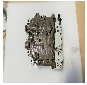
17. Some TCMs may not come with the Cutch Pressure Sensor Plate installed. This will require you to swap the CP plate from your existing TCM to the new 0301 TCM. To remove the plate, use your finger to push down on the tab in the photo and pull the plate up and to the left to release it from the tabs. **This should not require excessive force to remove or install.**
