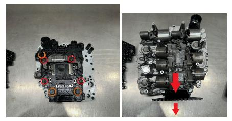
16. Carefully split the TCM from the mechatronic, taking note of the orientation of the unit. The 0301 TCM will need to be placed in the same orientation.
