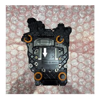
18. Place the clutch pressure sensor plate onto the 0301 TCM by first sliding in the right side of the plate under the tab shown in the photo below, then push into place, ensuring that the plate clips in and is 100% seated
