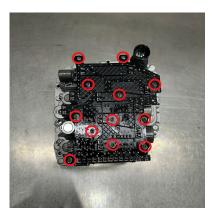
15. Use a T30 Torx to remove the four (4) fasteners holding the TCM to the mechatronic. The connector portion can be flipped out to clear the mechatronic when being removed.
