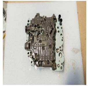
17. Place the new 0301 TCM on the mech unit and use the four (4) fasteners that were removed to secure the TCM to the mech. The fasteners are different lengths, take not of the position and replace them in the same orientation.
