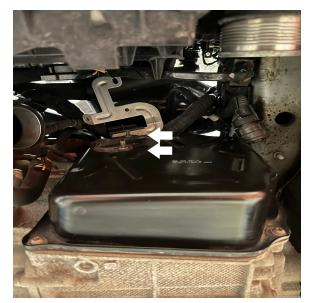
8. Remove the Mechatronic retainer clip. This may be easier from the top of the vehicle with the airbox removed.
