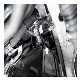
7. Using a 10mm socket, remove the two (2) fasteners that hold the harness bracket to the front of the Mechatronic pan and move the bracket out of the way.
